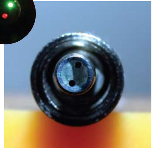
Reflectance probe, 2 fibers inside SMA connector
